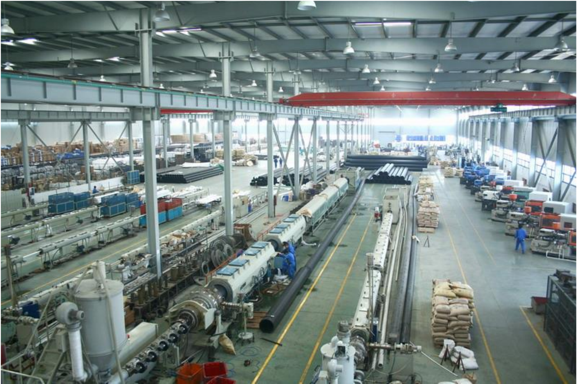
Production of plastic pipes by extrusion
